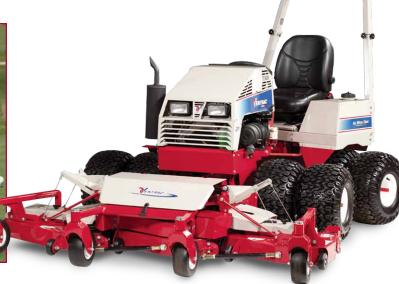
Ventrac's **Contour Mower** features a 83-inch working width making quick work of any mowing job regardless of the terrain without sacrificing quality of cut. Three independent decks aided by front rollers float along the contour of the ground
